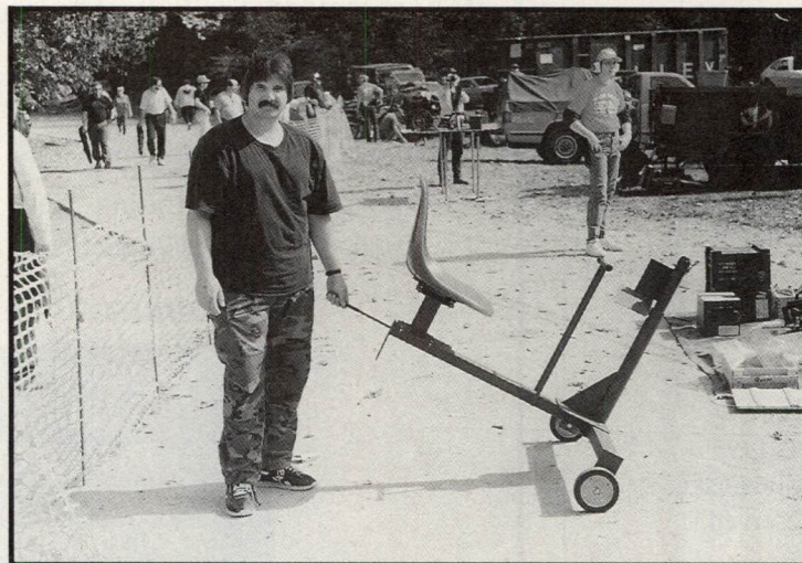
Fitted with optional "travel trolley" wheels, the MB94A1 machine gun mount is easily transportable.
