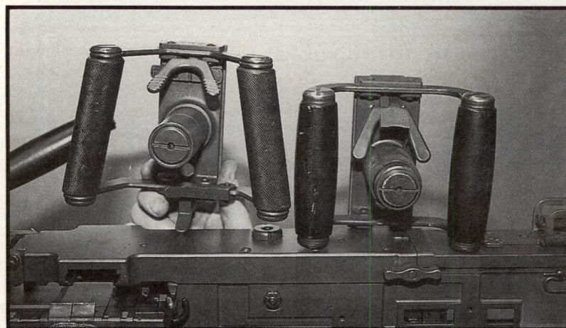
Comparison of new Fifty/.50 spade grips (left) and original M2 grips right.
